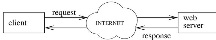
Figure 1: Interaction between client and web server
