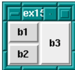
grid Geometry Manager, Cells With Sticky Edges
