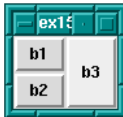
grid Geometry Manager, Cells With Sticky Edges
