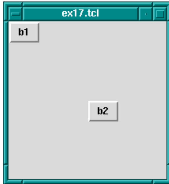
Using The place Geometry Manager
